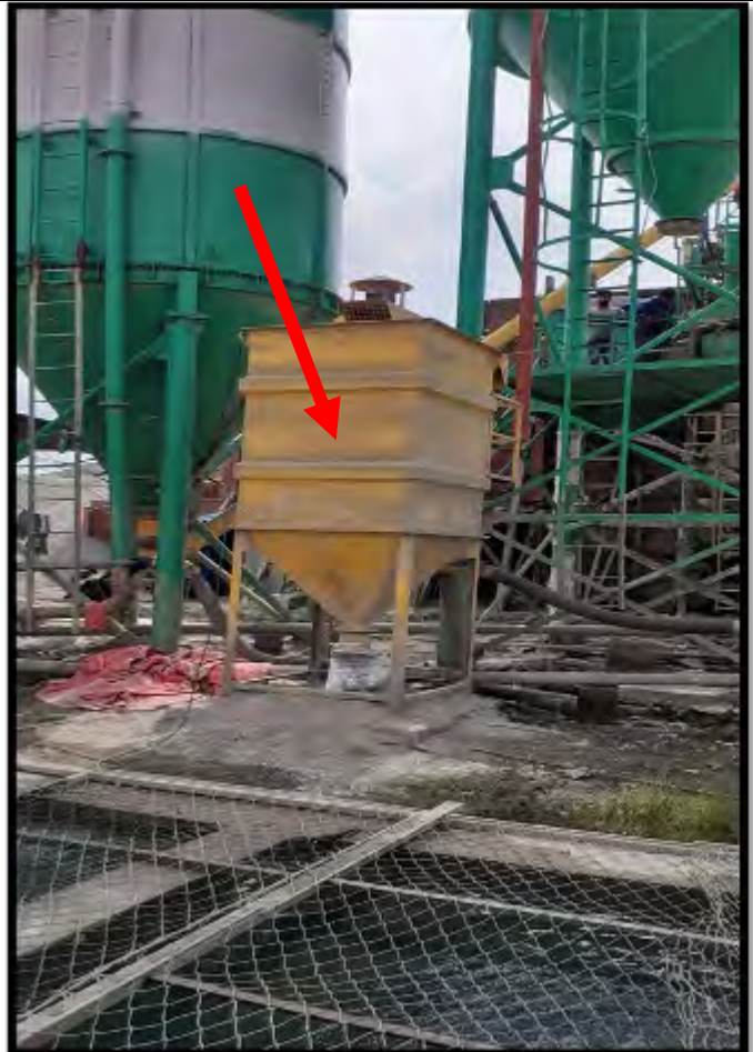
Dust collectors/Dust filter provided with cellos of batching plant to protect air pollution
