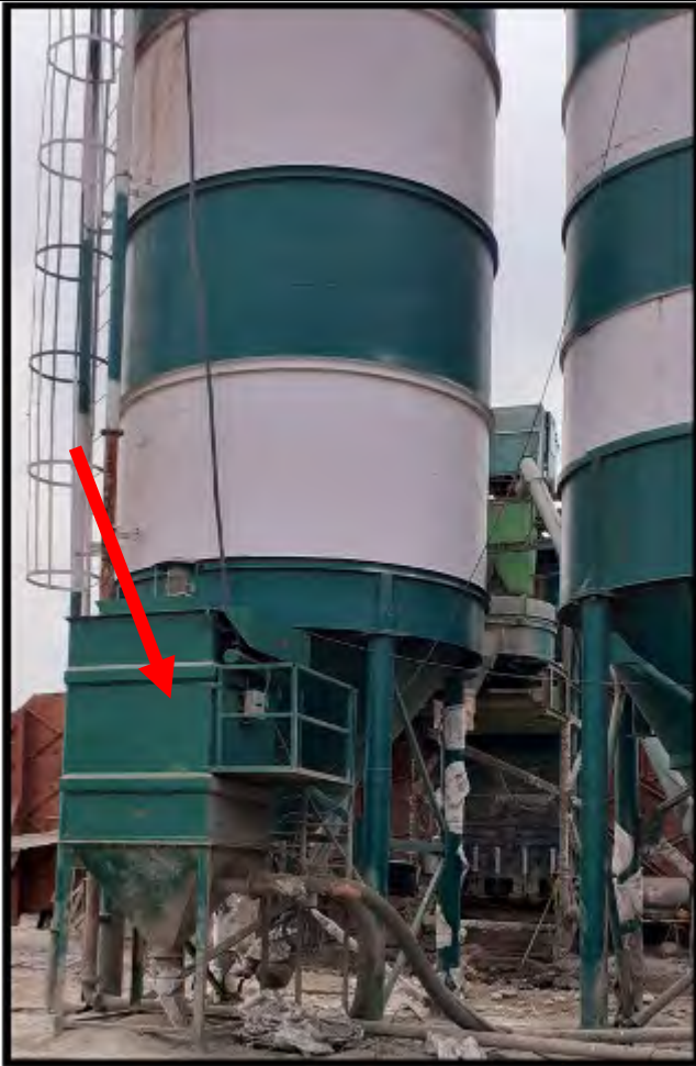
Dust collectors/Dust filter provided with cellos of batching plant to protect air pollution
