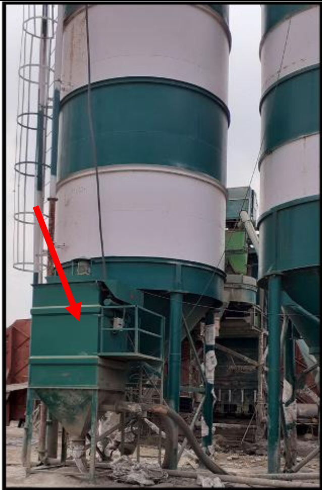
Dust collectors/Dust filter provided with cellos of batching plant to protect air pollution
